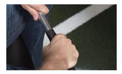
To ensure the rubber tip is pushed flush onto the metal pipe, first visually check to observe no adhesive is showing. The rubber tip should cover the adhesive. Finally, while seated in a chair, with one hand grab the top of the rubber tip and with the other hand the lower metal pipe. Place the tee horizontally between your legs and use arms and legs together to firmly push inward. This ensures the rubber tip is flush.
